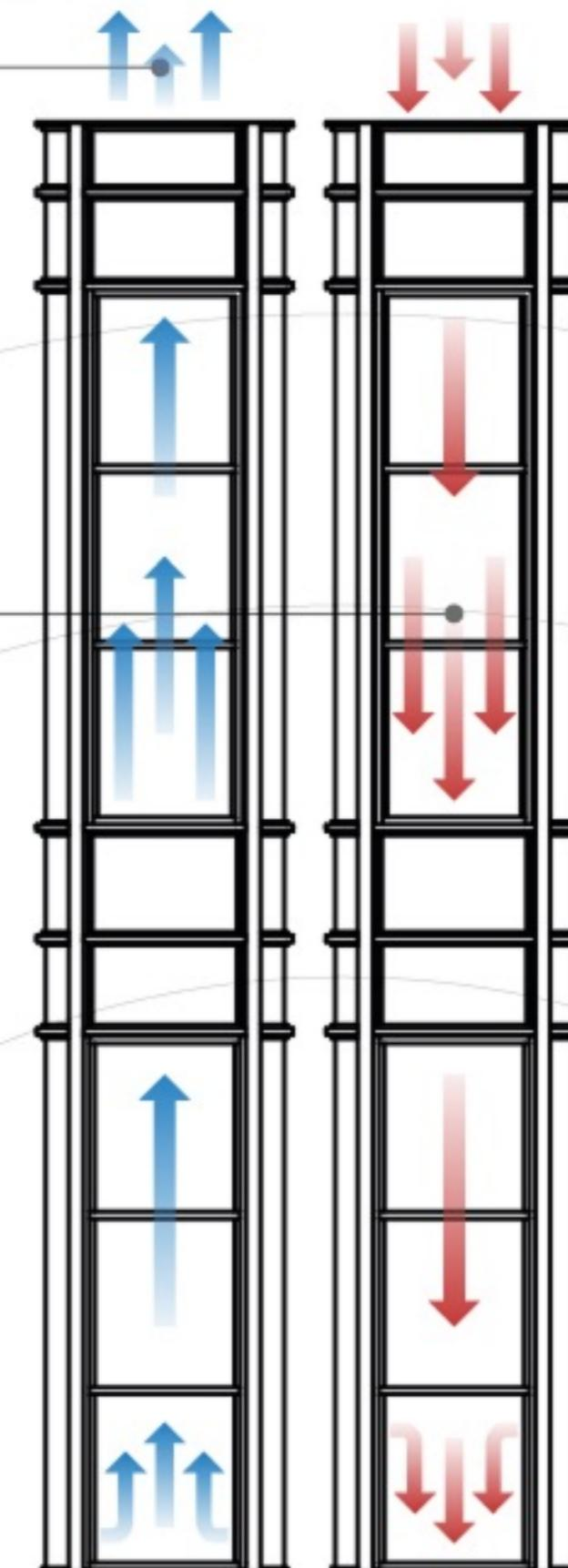
For descent, the air intake is controlled, lowering the cabin gently with minimal power consumption.
